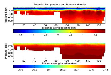
**Figure 7**. Data collected by the British glider, which complements an offshore LTER glider. In the potential temperature the eddies of modified circumpolar deep water is visible as warm water present between 200 and 400 meter water depth.
